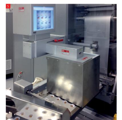
Pic. 1) Camera housing with LEDs
